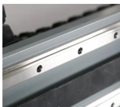
Linear guide & synchronous belt
